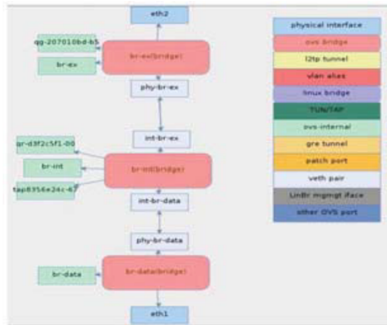
Figure 6. Network elements within an OpenStack network node [13].
